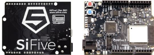
Figure 2: HiFive1 Rev B01 board (top and bottom view)
